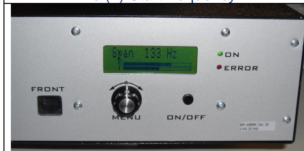
Span (=) Frequency span
